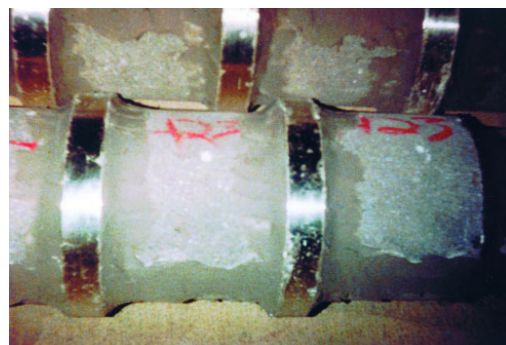
Fig. 13 — Tunnel furnace rolls re-insulated with preformed shapes.
