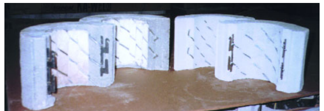
Fig. 6 — Preformed refractory shapes.
