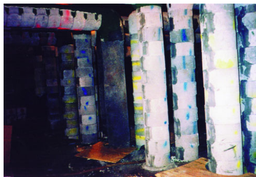
Fig. 14 — Color coding of preformed shapes.
