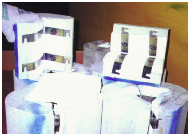
Fig. 8 — View of a composite shape before installation, showing the fiber layer adjacent to the pipe being surrounded by a hard refractory outer shell.
